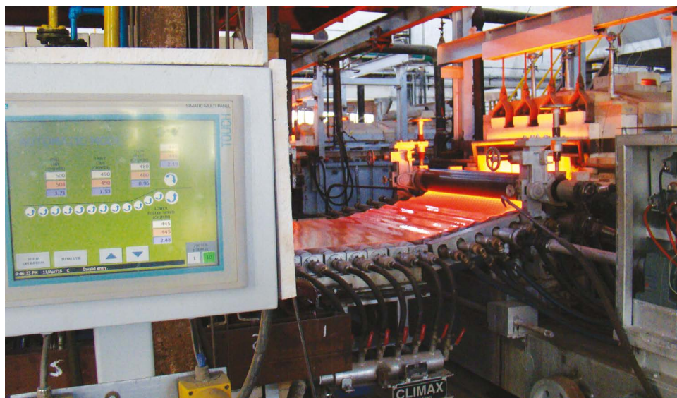
The rolled glass process at Gopal Glass Works.
